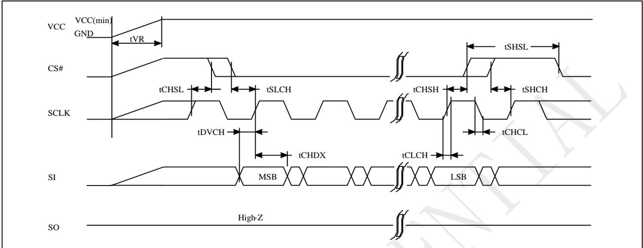
**Figure 5-9 Power-up Timing**
