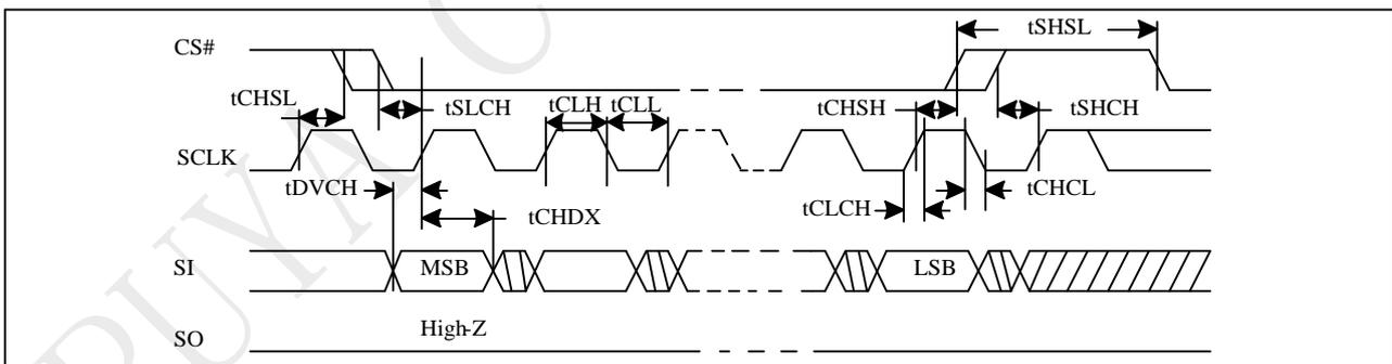
Figure 5-5 Output Timing
