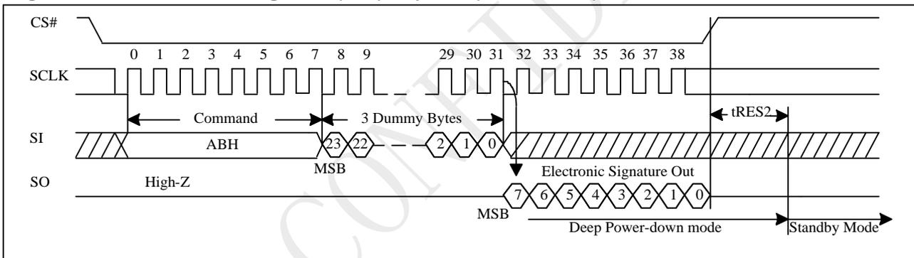
Figure 10-39a Read Electronic Signature (RES) Sequence (QPI)
