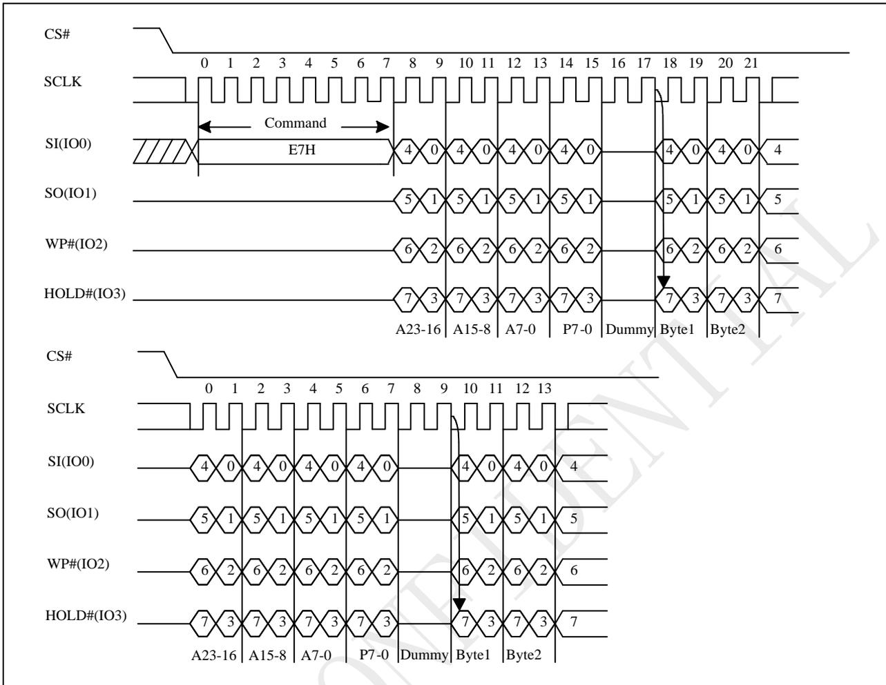
**4 X I/O Word Read with “8/16/32/64-Byte Wrap Around” in Standard SPI mode**
