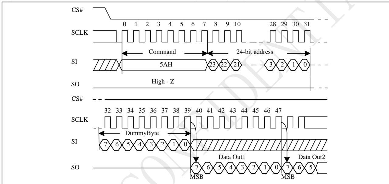
Figure 10-56a Read Serial Flash Discoverable Parameter (RDSFDP) Sequence(QPI)
