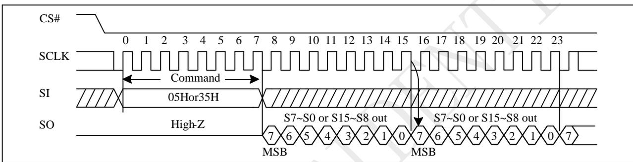
**Figure 10-5a Read Status Register (RDSR) Sequence (QPI)**
