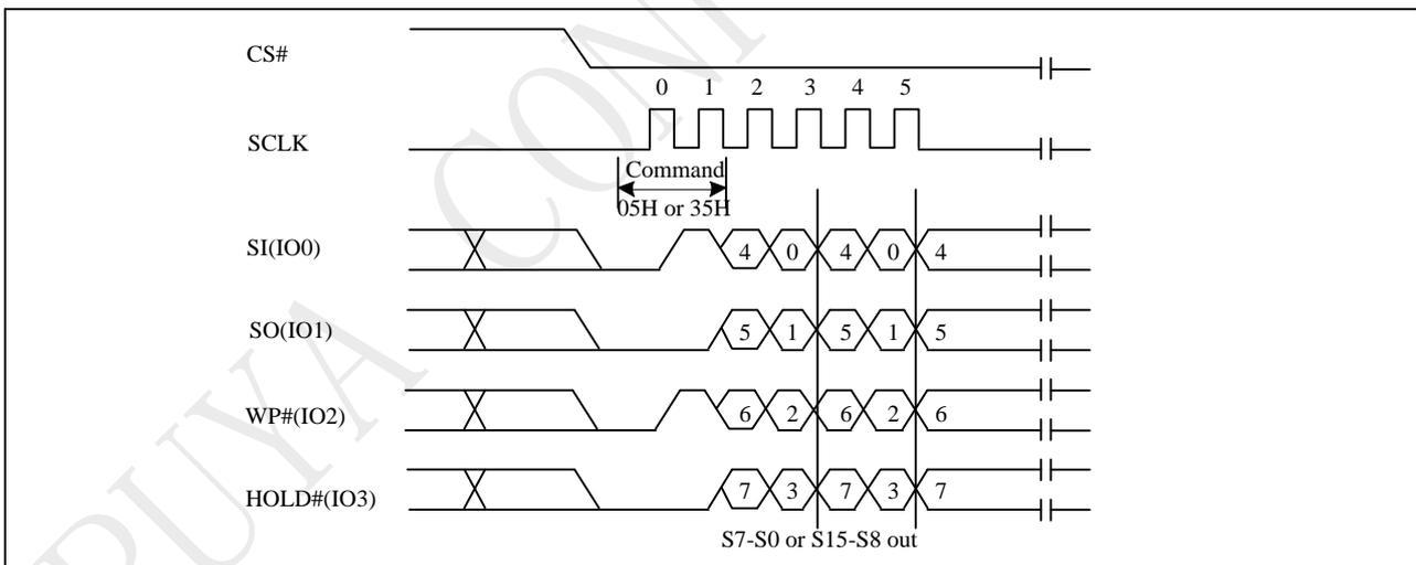
Figure 10-5b Read Status Register (RDSR) Sequence (QPI)
