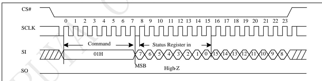
Figure 10-8a Write Status Register (WRSR) Sequence (QPI)
