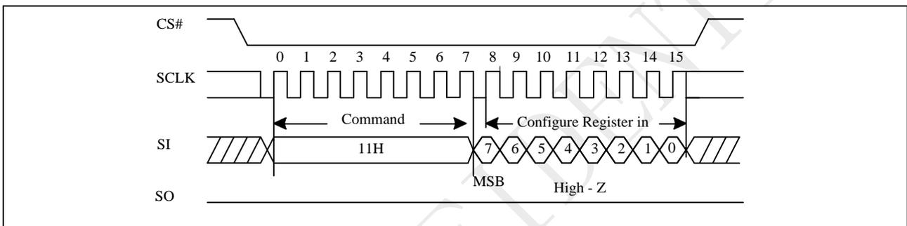
Figure 10-9a Write Configure Register (WRCR) Sequence (QPI)
