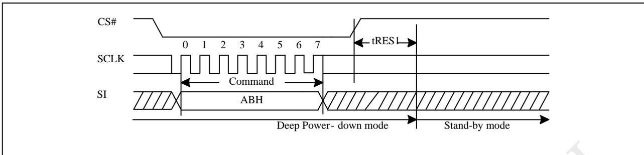
Figure 10-39c Release from Deep Power-down (RDP) Sequence (QPI)
