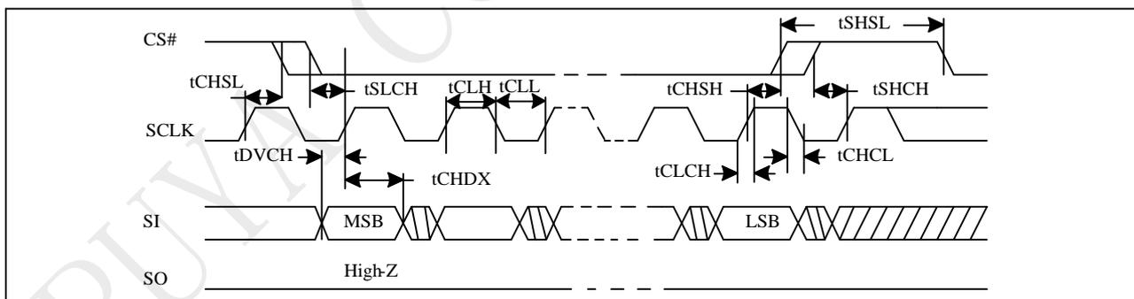
Figure 5-5 Output Timing
