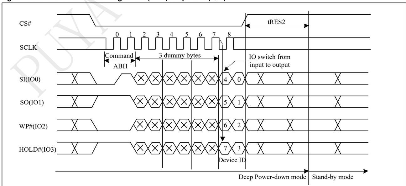
**Figure 10-53b Release from Deep Power-down (RDP) Sequence (Command ABH)**
