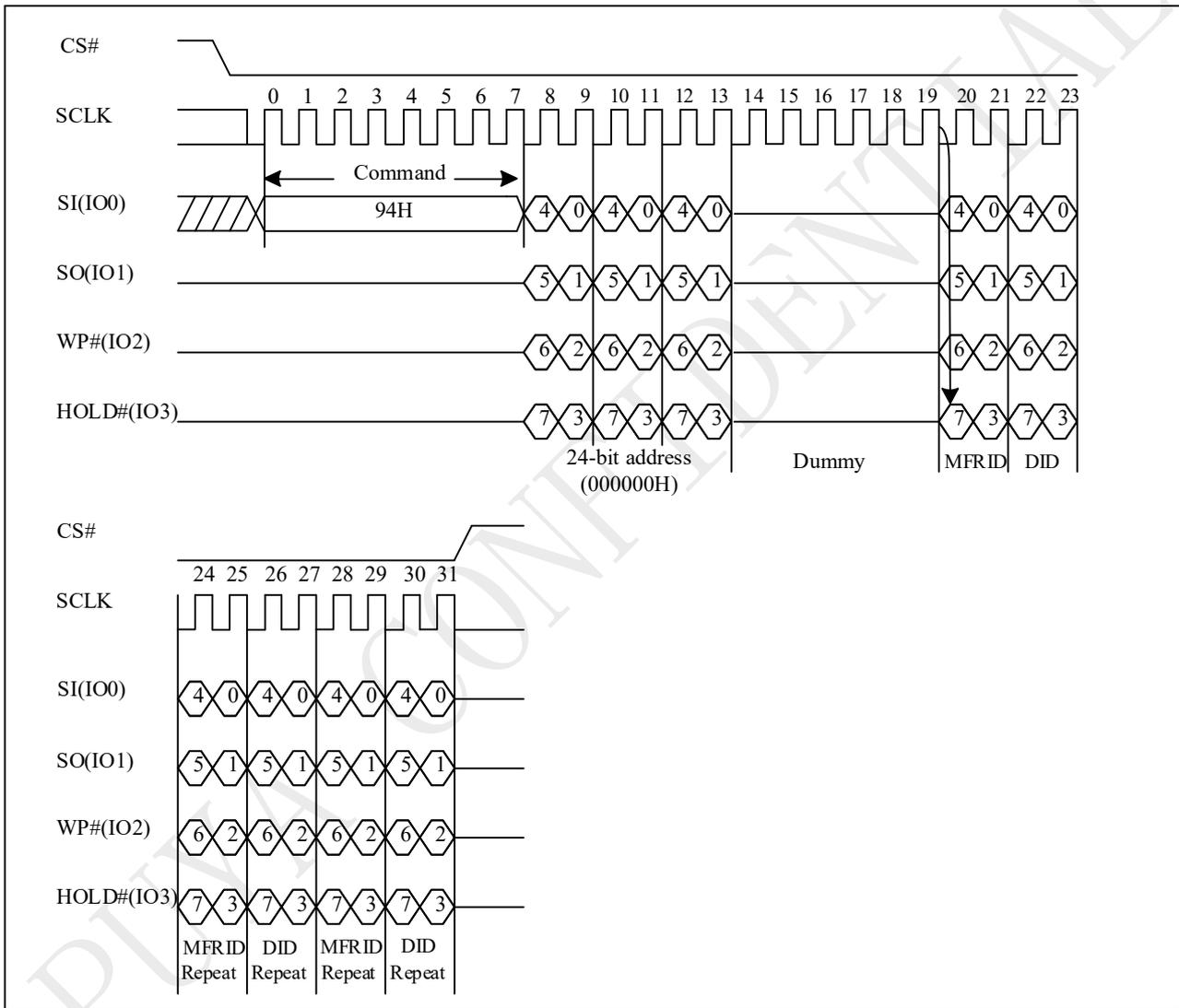
Note: 32-bit address (0000\_0000H) are required when the device is operation in 4-byte address mode.
