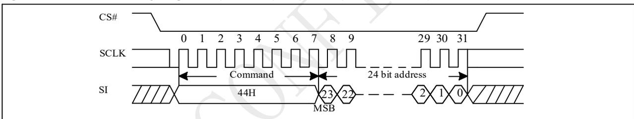
Figure 10-49a Erase Security Registers (ERSCUR) Sequence (QPI 44H)
