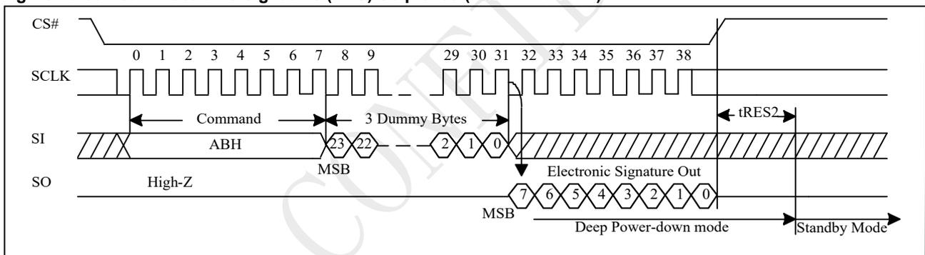
**Figure 10-53a Read Electronic Signature (RES) Sequence (QPI)**
