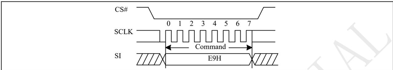
**Figure 10-12a Exit 4-Byte Address Mode Sequence (QPI)**
