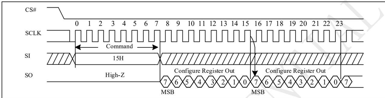
Figure 10-6a Read Status Register (RDCR) Sequence (QPI)
