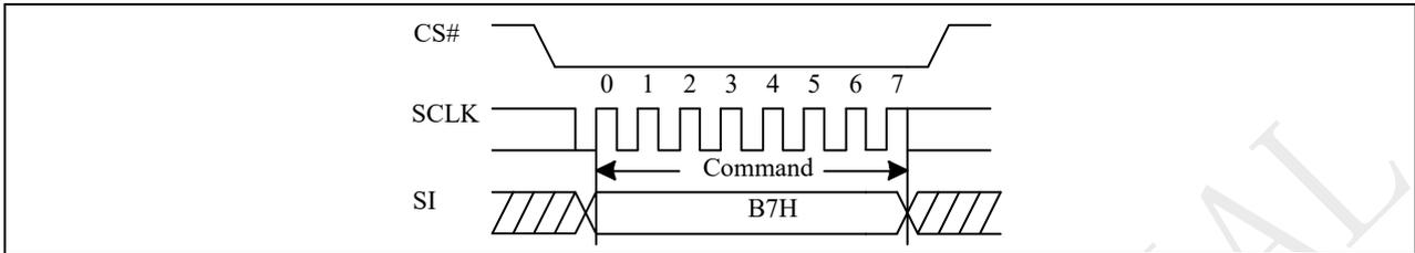
Figure 10-11a Enter 4-Byte Address Mode Sequence (QPI)
