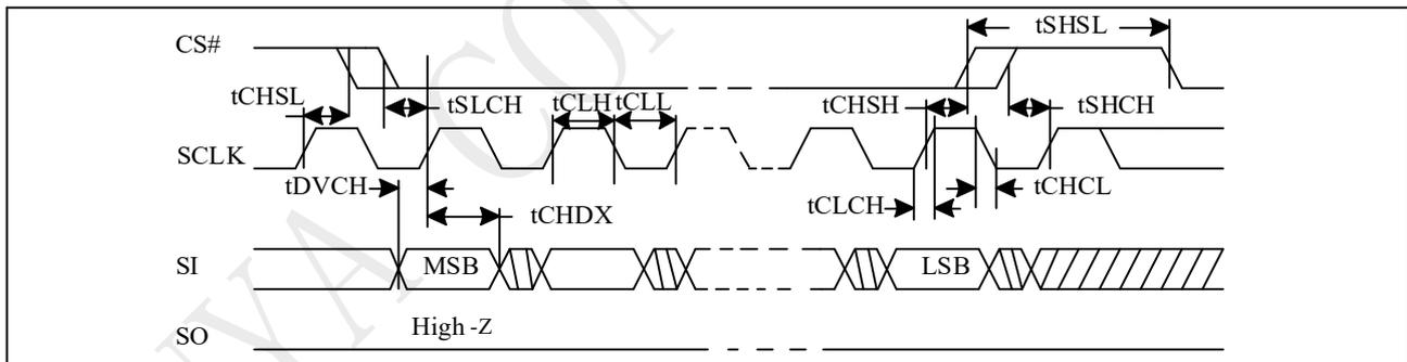
Figure 5-5 Output Timing
