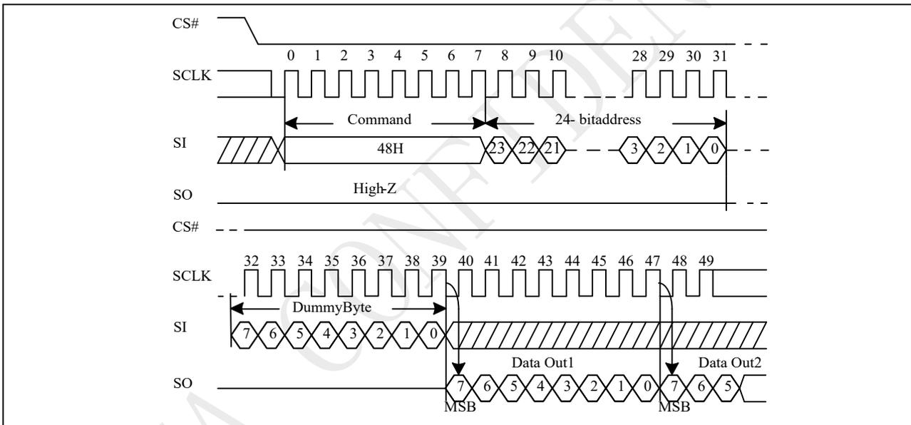
Figure 10-51a Read Security Registers (RDSCUR) Sequence (QPI 48H)
