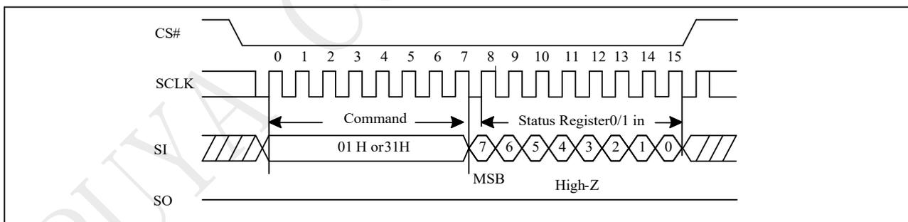
**Figure 10-7a Write Status Register (WRSR) Sequence (QPI)**
