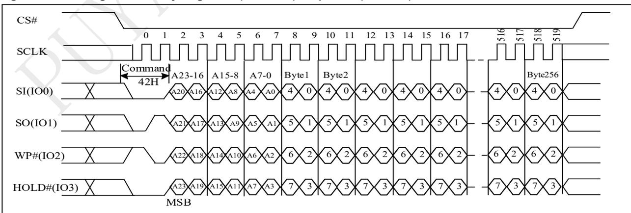
Note: 32-bit address is required when the device is operation in 4-byte address mode.
