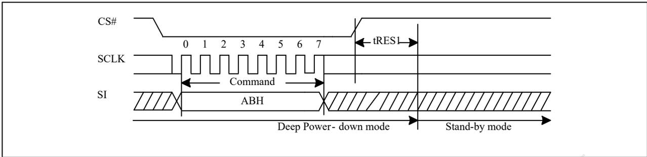
**Figure 10-53c Release from Deep Power-down (RDP) Sequence (QPI)**
