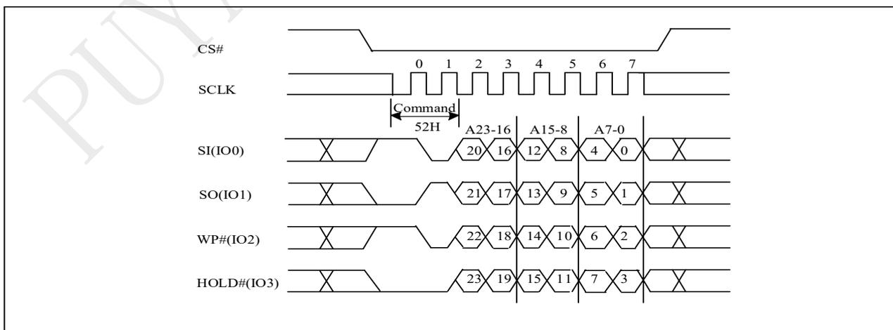
Note: 32-bit address is required when the device is operation in 4-byte address mode.
