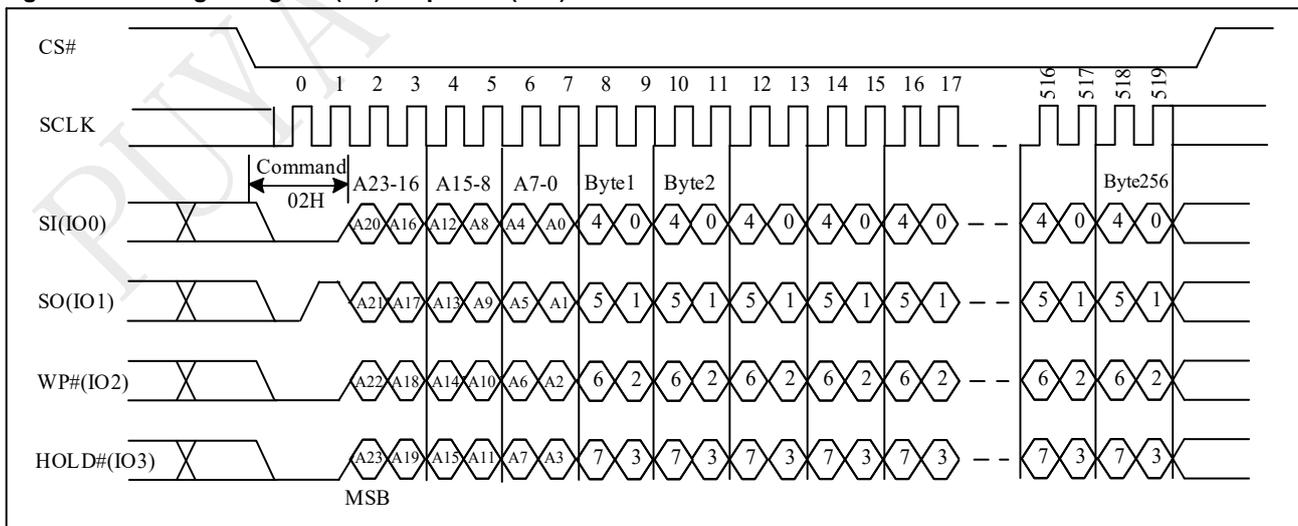
Note: 32-bit address is required when the device is operation in 4-byte address mode.
