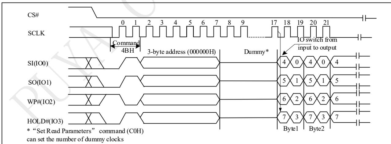
Note: 4 bytes address 0000\_0000H is required when the device is operation in 4-byte address mode.
