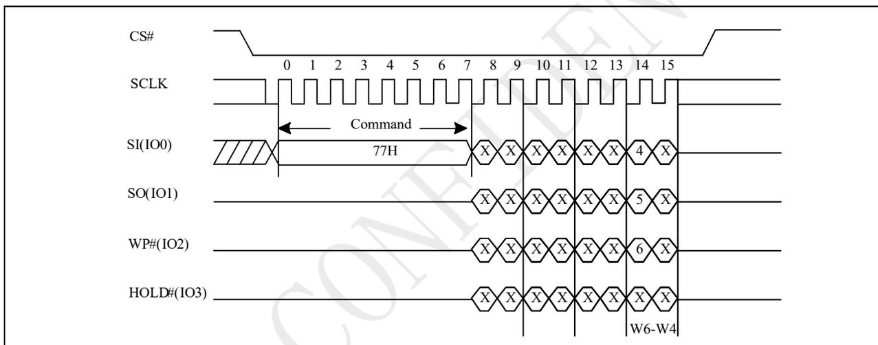
Note: 32-bit dummy bits are required when the device is operation in 4-byte address mode.
