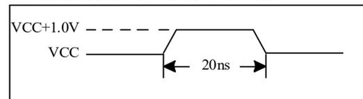
During DC conditions, input or I/O signals should remain equal to or between V<sub>SS</sub> and V<sub>CC</sub>. During voltage transitions, inputs or I/Os may negative overshoot to -1.0V or positive overshoot to V<sub>CC</sub> + 1.0 V, for periods up to 20 ns.
