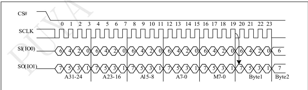
Note: 2IO Continue Read with 4-Byte Address, if M5-4 = 1, 0. If not using Continue Read recommend to set M5-4 ≠ 1, 0.
