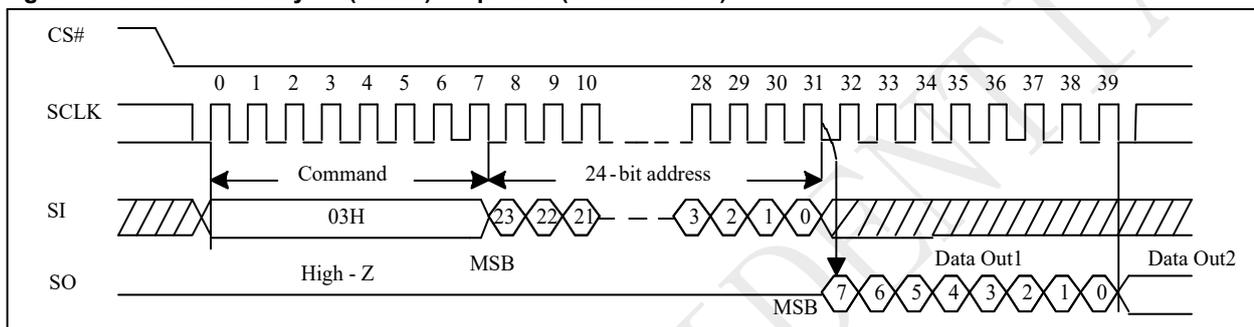
Note: 32-bit address is required when the device is operation in 4-byte address mode.
