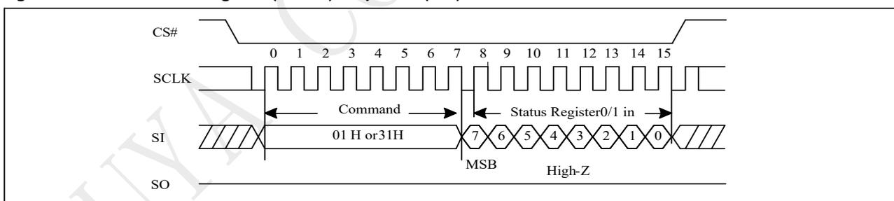
**Figure 10-7a Write Status Register (WRSR) Sequence (QPI)**
