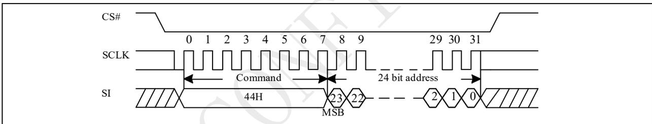
Figure 10-46a Erase Security Registers (ERSCUR) Sequence (QPI)
