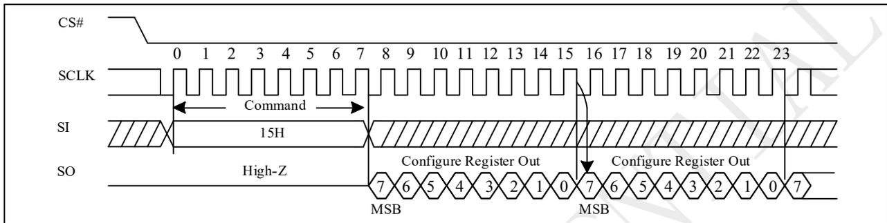
**Figure 10-6a Read Status Register (RDCR) Sequence (QPI)**
