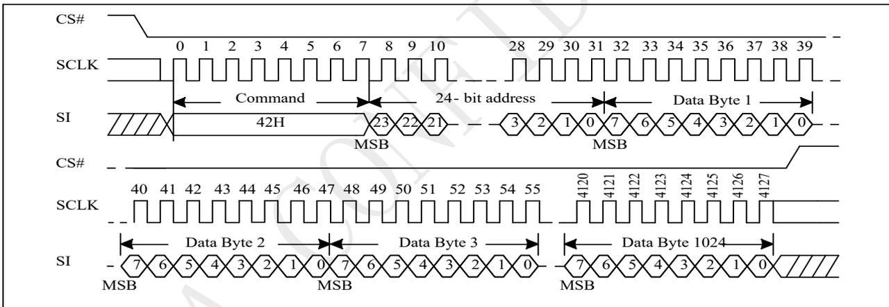
Figure 10-47a Program Security Registers (PRSCUR) Sequence (QPI)
