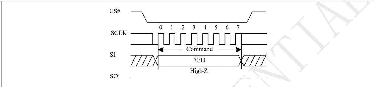
**Figure 10-62a Global Block Lock (QPI)**
