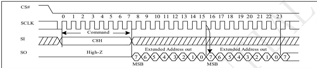
**Figure 10-9a Read Extended Address Register Sequence (QPI)**
