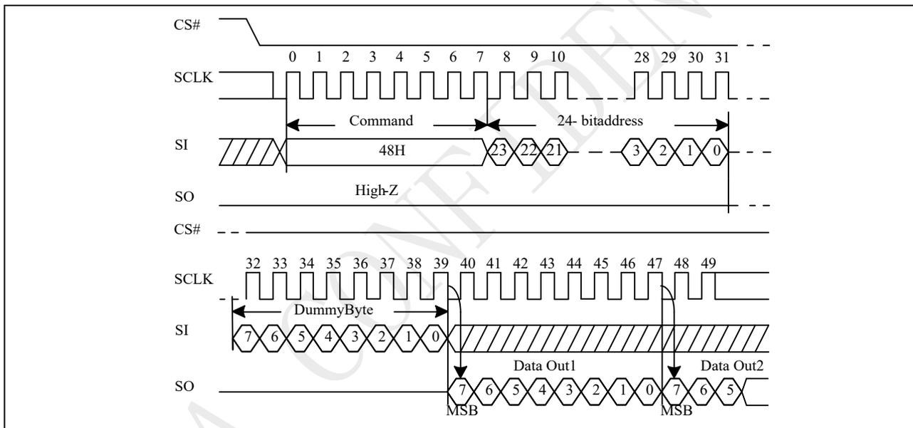
Figure 10-48a Read Security Registers (RDSCUR) Sequence (QPI)
