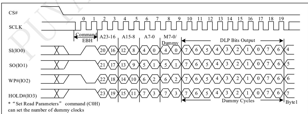
**Figure 10-30g DTR 1IO Read with DLP bits output Sequence (SPI)**
