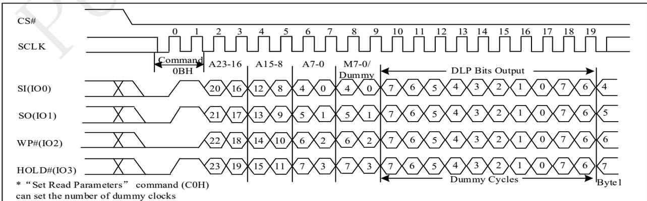
**Figure 10-30b Dual Read with DLP bits output Sequence (SPI)**
