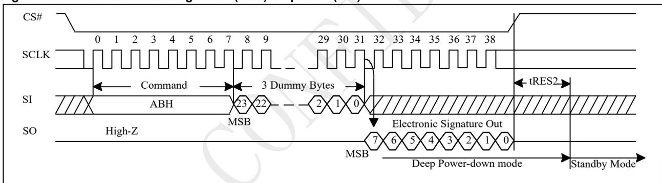
**Figure 10-50a Read Electronic Signature (RES) Sequence (QPI)**
