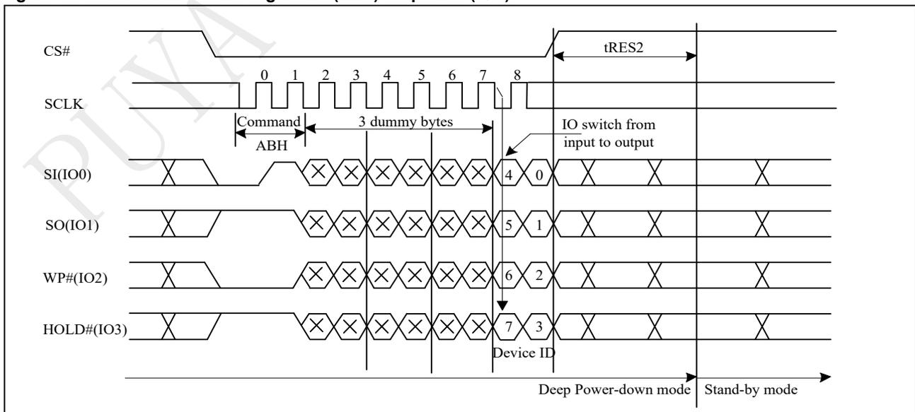
**Figure 10-50b Release from Deep Power-down (RDP) Sequence (SPI)**
