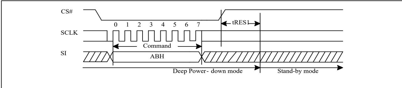
**Figure 10-50c Release from Deep Power-down (RDP) Sequence (QPI)**
