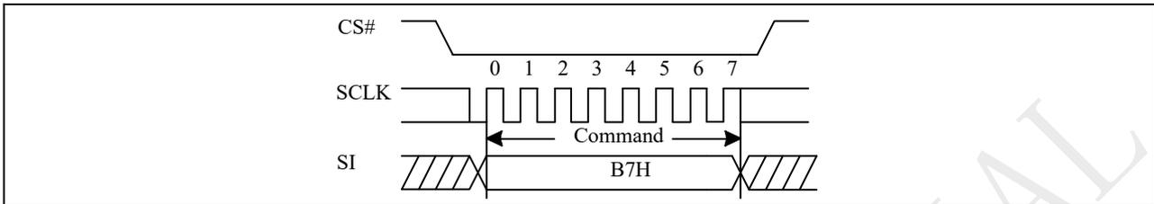
Figure 10-11a Enter 4-Byte Address Mode Sequence (QPI)
