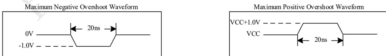
During DC conditions, input or I/O signals should remain equal to or between VSS and VCC. During voltage transitions, inputs or I/Os may negative overshoot to -1.0V or positive overshoot to VCC + 1.0 V, for periods up to 20 ns.
