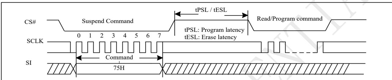
**Figure 10-42a Suspend to Read/Program Latency (QPI)**
