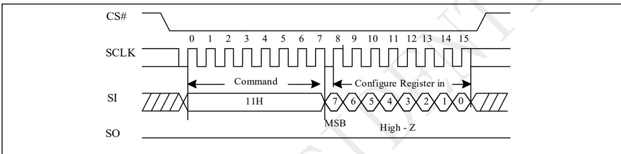
**Figure 10-8a Write Configure Register (WRCR) Sequence (QPI)**
