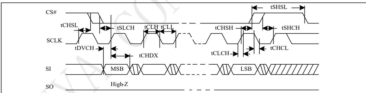
Figure 5-5 Output Timing
