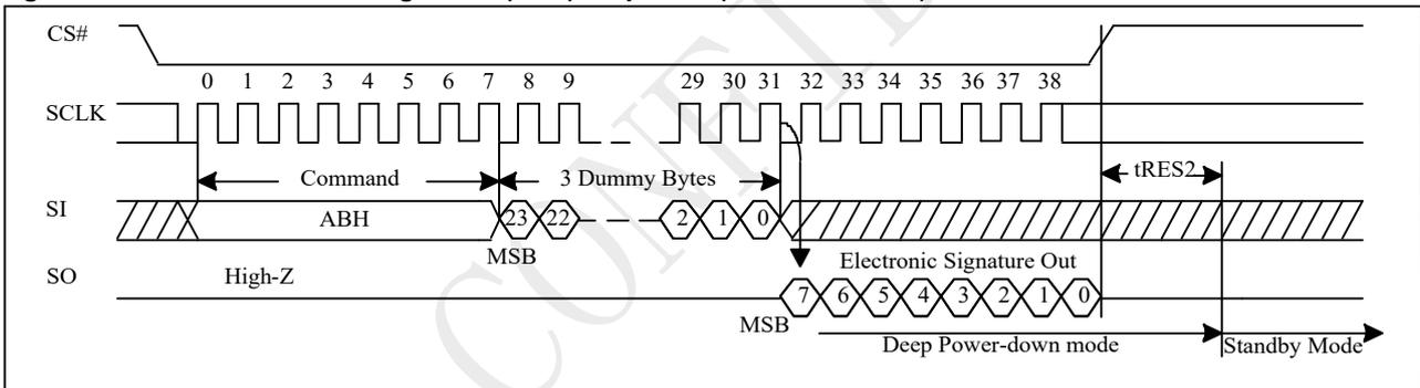
**Figure 10-36a Read Electronic Signature (RES) Sequence (QPI)**
