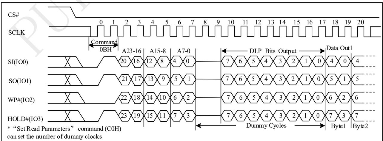
**Figure 10-23b Dual Read with DLP bits output Sequence**
