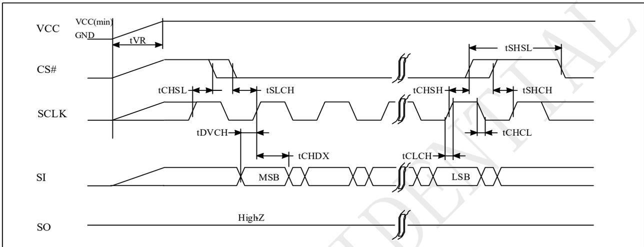
Figure 5-9 Power-Up Timing
